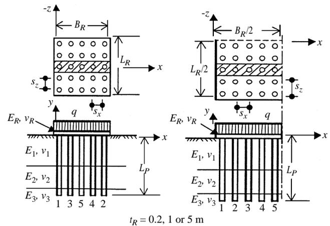
Fig. 2 Typical piled raft configurations for numerical analysis
