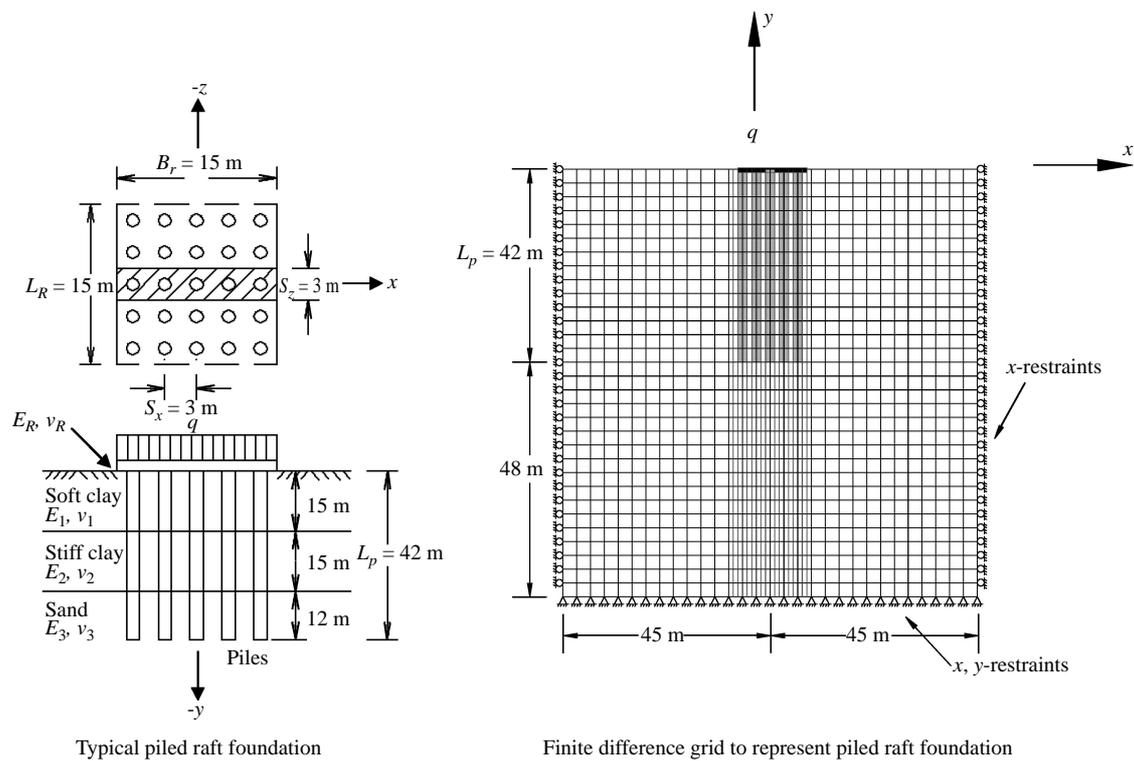
Fig. 1 Typical finite difference discretization of piled raft system
