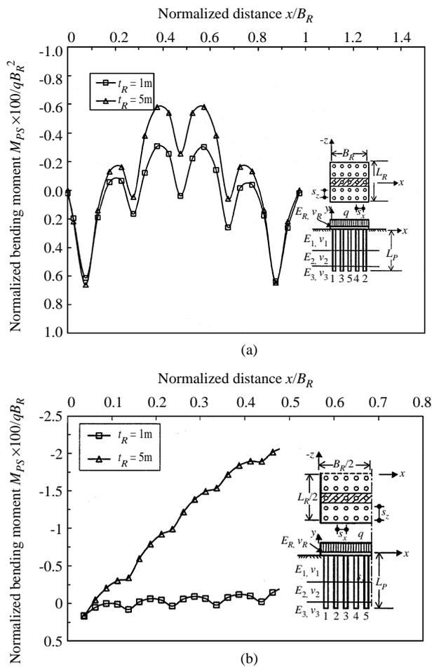
Fig. 5 (a) Bedding moment of piled raft with dimensions  $B_R \times L_R = 15\text{ m} \times 15\text{ m}$  ( $5 \times 5$  piles), raft edge-to-raft edge plot. (b) Bending moment in piled raft with dimensions  $B_R \times L_R = 30\text{ m} \times 30\text{ m}$  ( $10 \times 10$  piles), raft edge-to-raft center plot.
