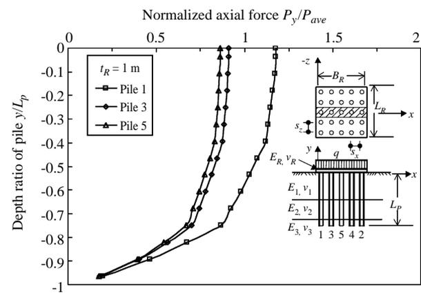
Fig. 7 (a) Axial force distribution in pile structure of piled raft with dimensions  $B_R \times L_R = 15\text{ m} \times 15\text{ m}$  ( $5 \times 5$  piles),  $L_p = 42\text{ m}$ ,  $q = 333\text{ kPa}$ .
