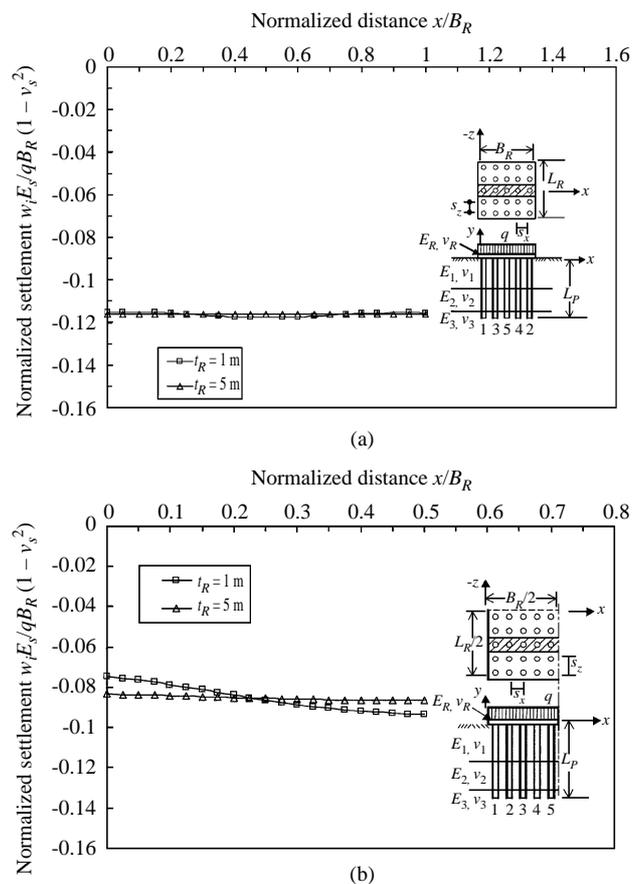
Fig. 3 (a) Normalized settlement of piled raft with  $B_R \times L_R = 15 \text{ m} \times 15 \text{ m}$  ( $5 \times 5$  piles) or different raft thicknesses, raft edge-to-raft edge plot. (b) Normalized settlement of piled raft with dimensions  $B_R \times L_R = 30 \text{ m} \times 30 \text{ m}$  ( $10 \times 10$  piles), raft edge-to-raft center plot.
