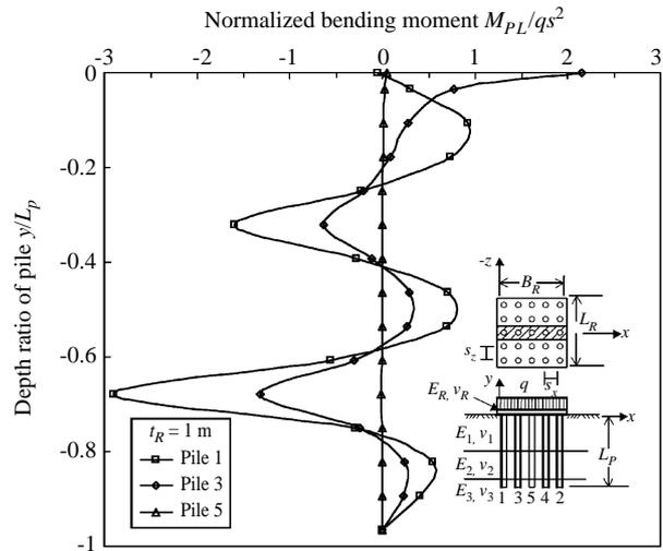
Fig. 8 Bending moment distribution in pile structure of piled raft with dimensions  $B_R \times L_R = 15 \text{ m} \times 15 \text{ m}$  ( $5 \times 5$  piles),  $L_p = 42 \text{ m}$ ,  $q = 333 \text{ kPa}$ .
