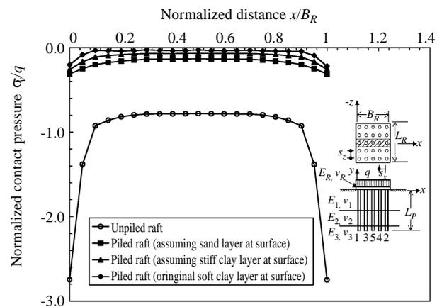
Fig. 6 Comparison of contact pressure at raft-soil interface among piled rafts and unpiled raft,  $t_R = 1\text{ m}$ , raft edge-to-raft edge plot
