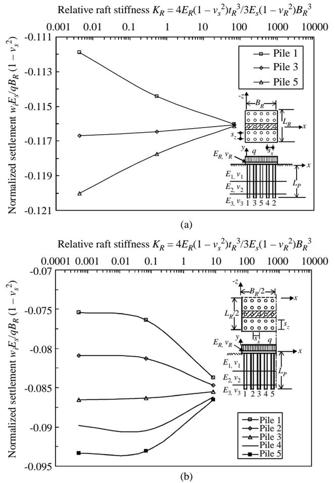
Fig. 4 (a) Effect of raft stiffness on settlement of piled raft with dimension  $B_R \times L_R = 15$  m  $\times$  15 m (5  $\times$  5 piles), raft edge-to-raft edge plot. (b) Effect of raft stiffness on settlement of piled raft with dimension  $B_R \times L_R = 30$  m  $\times$  30 m (10  $\times$  10 piles), raft edge-to-raft center plot.
