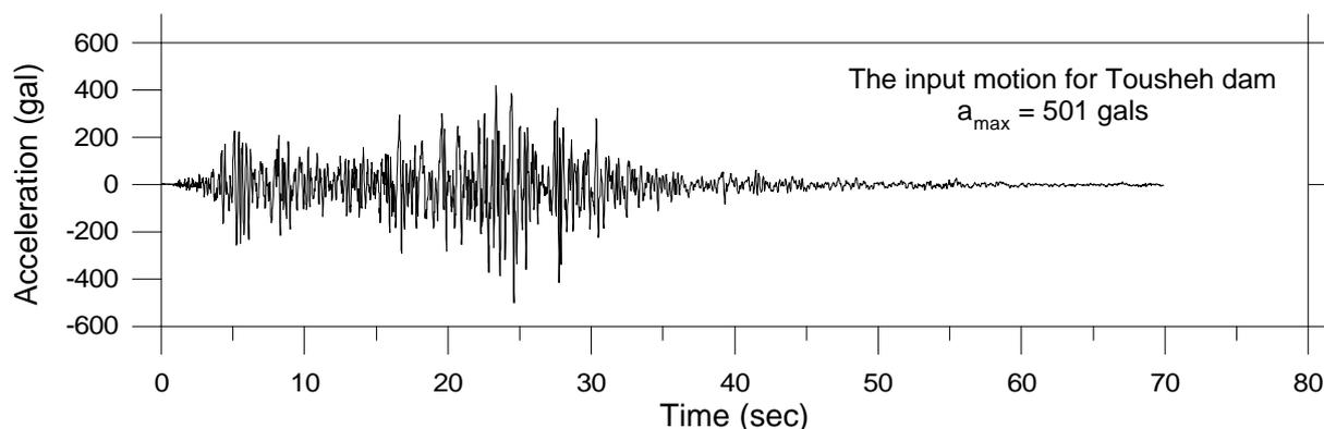
Figure 3. The Chi-Chi earthquake input motion for Tousheh dam
