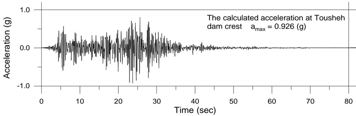
Figure 4 The acceleration response at the dam crest
