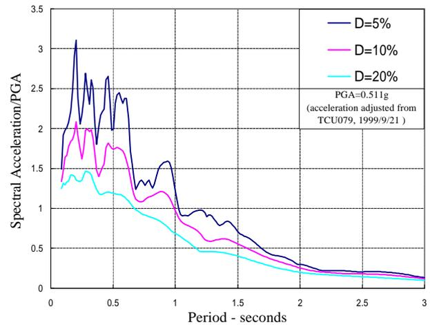
Figure 8. The response spectra for Tousheh dam
