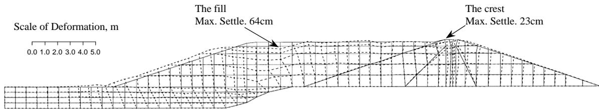
Figure 6. Estimated permanent deformation of Tousheh dam after Chi-Chi earthquake
