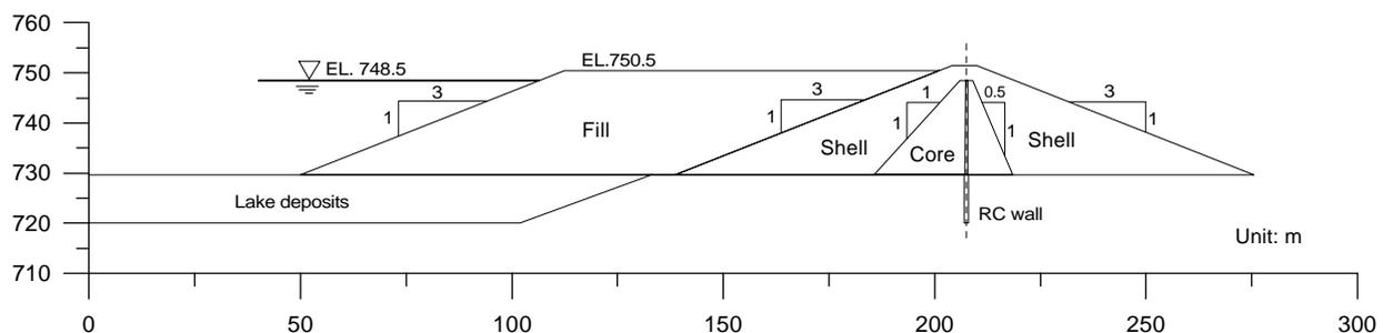
Figure 1. A typical section of Tousheh dam
