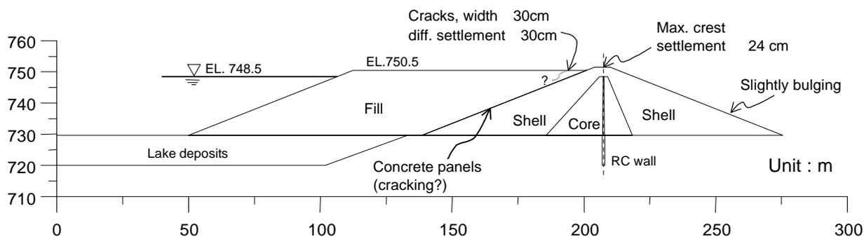
Figure 2. Measured settlements and locations of cracks after Chi-Chi earthquake
