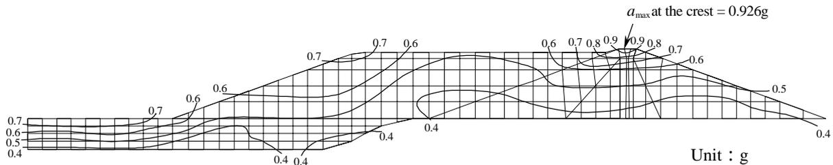
Figure 5. The contour plot of peak accelerations of Tousheh dam during Chi-Chi earthquake
