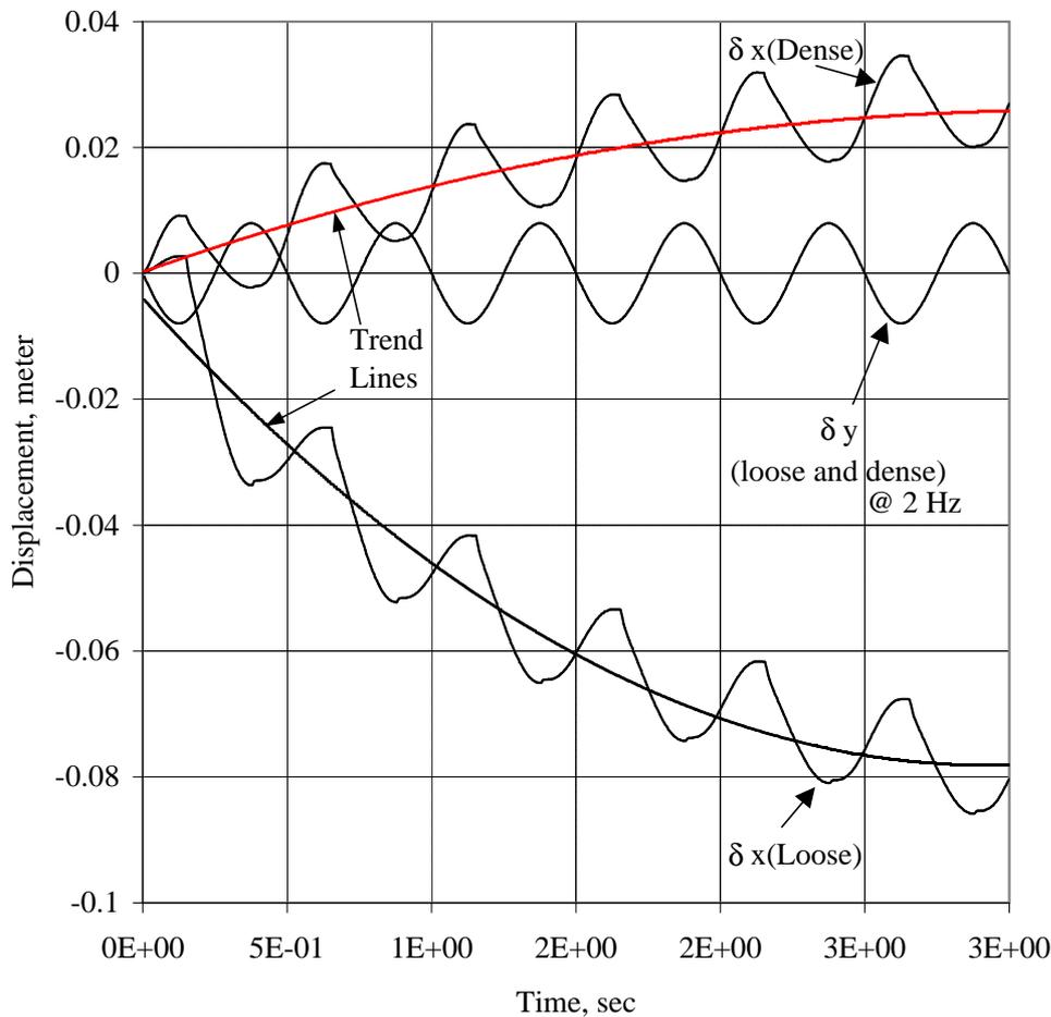
Figure 5 Lateral displacements ( $\mathbf{dx}$ ) versus time in response to the same imposed cyclic axial displacements ( $\mathbf{dy}$ ) for loose and dense soil elements (Leonards et al, 1995).
