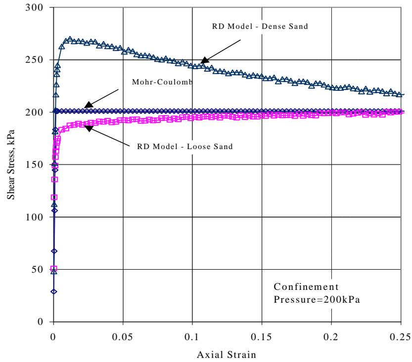
Figure 2 Stress versus strain curves of the triaxial compression tests on the soil models for the circular foundation simulations.
