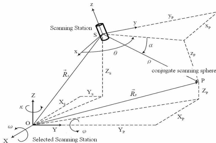
Fig. 4 The spatial coordinate relationship between scanning stations and conjugate scanning spheres ( modified from Lichti, 2002 )
