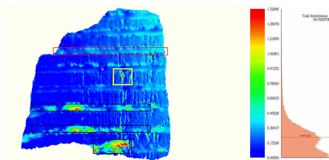
Fig. 14 The surface variation result after overlapping the two scanned data sets.
