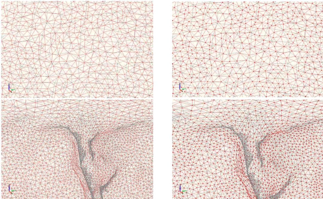
Fig. 12 Overlapping TIN model for a flat zone (upper left); vertices of triangles of the first scanning TIN surface for a flat zone (upper right); Overlapping TIN model for a undulate zone (lower left); vertices of triangles of the first scanning TIN surface for a undulate zone (lower right). Note: The first scanning TIN is shown in red color, and the second scanning TIN in grey.
