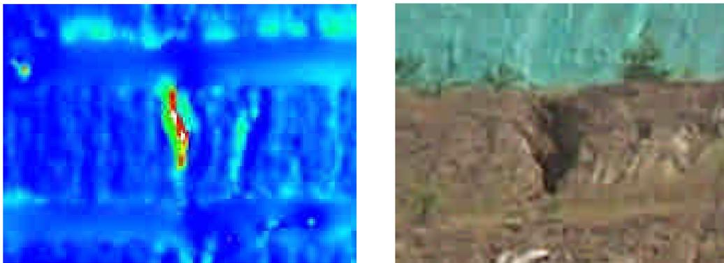
Fig. 16 The sliding area revealed by the second scanning and overlapping (left); the site photo of the sliding area.
