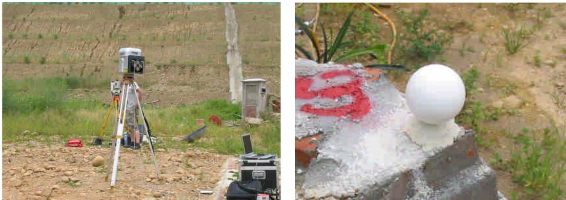
Fig.3 Scanning station and the 3D scanner (left) and one of the conjugate scanning spheres (right).
