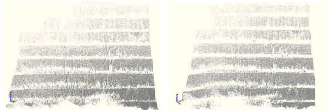
Fig. 8 3D point-cloud data from the first scanning (left) and the second scanning (right)
