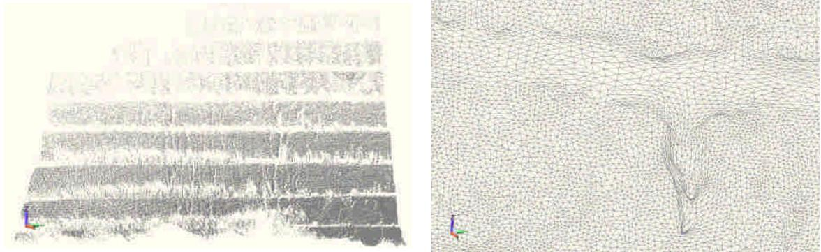
Fig. 5 The 3D point-cloud data (left); the surface model composed using TIN (right).
