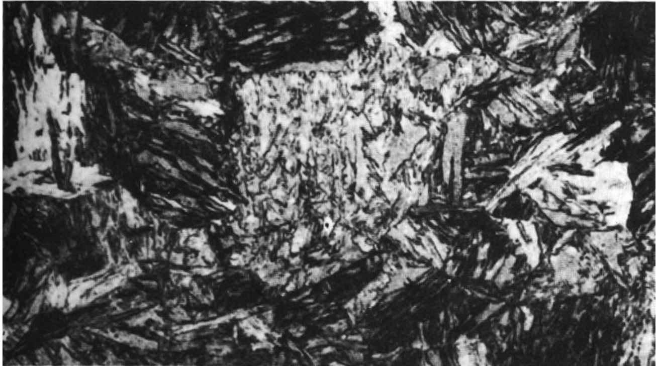
Figure 10-13 Acicular, or needlelike, microstructure of martensite 1000 \times . (From Metals Handbook, 8th Ed., Vol. 7: Atlas of Microstructures, American Society for Metals, Metals Park, Ohio, 1972.)
