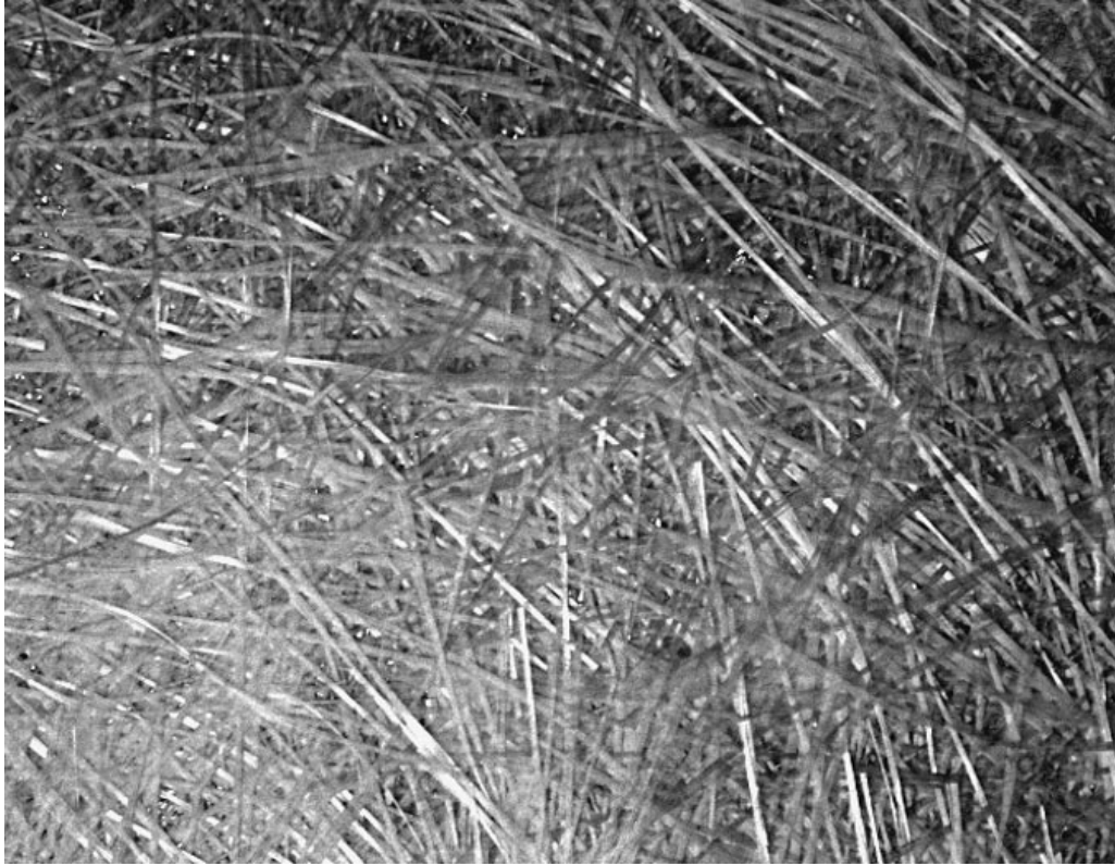
Figure 14-1 Glass fibers to be used for reinforcement in a fiber-glass composite. (Courtesy of Owens-Corning Fiberglas Corporation)
