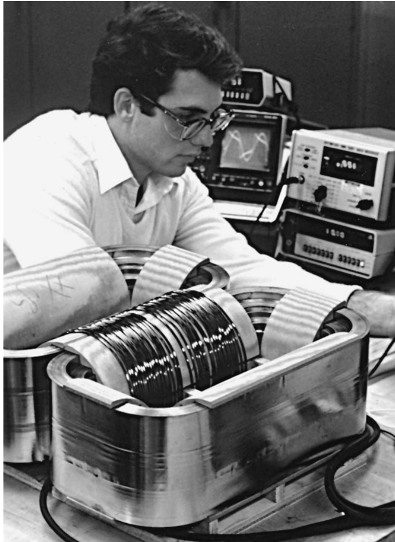
Figure 20-17 Transformer core winding using an amorphous ferrous alloy wire. (Courtesy of Allied-Signal, Inc.)
