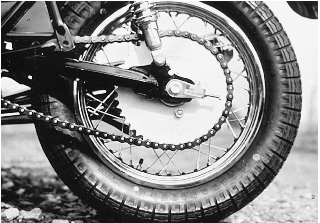
Figure 20-7 A drive sprocket made from dispersion-toughened nylon has replaced aluminum and steel parts in many motocross racing designs. (Courtesy of the Du Pont Company, Engineering Polymers Division)
