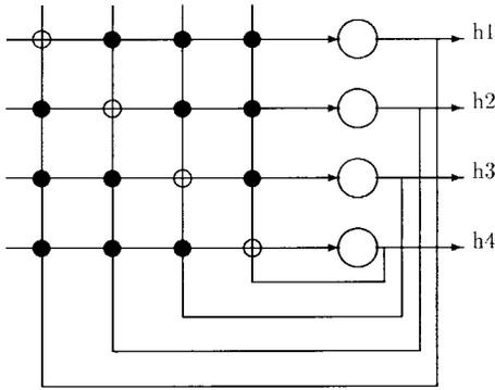
Fig. 2. The network architecture of the proposed WTA neural network. The hollow circles correspond to excitatory connections while the solid black circles correspond to inhibitory connections.
