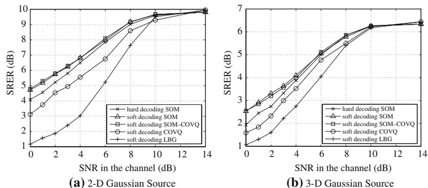
**Fig. 6** The signal-to-reconstruction error ratio (SRER) in dB. The channel is a fading channel
