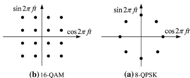
**Fig. 1** Two modulation methods. **a** QPSK and **b** QAM
